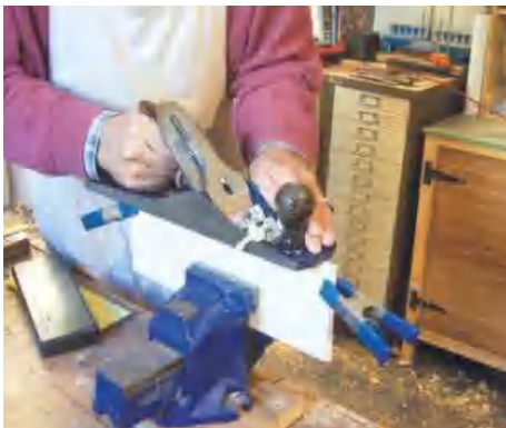
STEP 21. Planing the inside edges of the maple back while clamped in the vice
